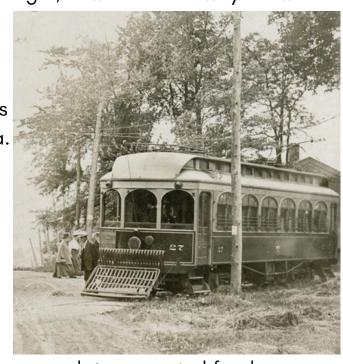
In 2005, the restoration was completed. A few years later, a period fender, a large metal grate on the front of the car designed so that animals wouldn't get run over, was reinstalled on the front of the car.
