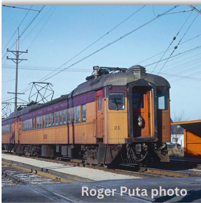
Car 24 was built in 1927 by the Pullman Car Company, and then began serving the railroad for over 55 years as a coach car. During the second World War, some of the cars, including 24, were modernized by increasing the length and capacity of the car due to increased ridership. A new interior was also put in, along with large sealed windows and air conditioning.
