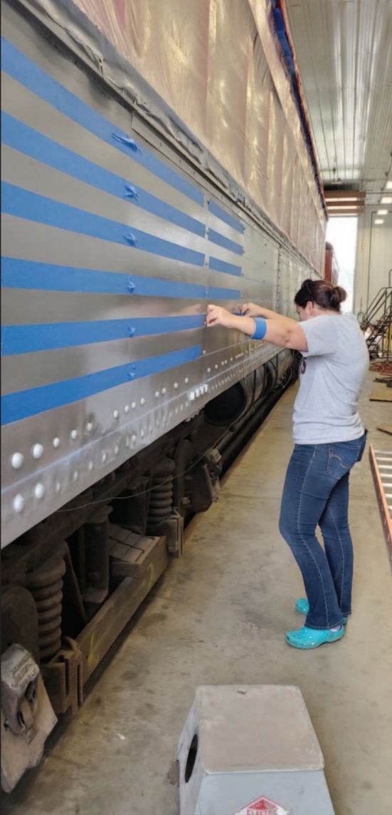
▲ Stephanie Zabelny applies the masking tape necessary to deliver the striping that will give the car a fluted stainless-steel appearance.
