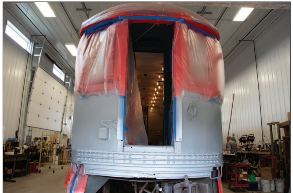
▲ The top of the car was wrapped in plastic and the bottom of the car had been painted with the grey base coat in this September 26th photo.
