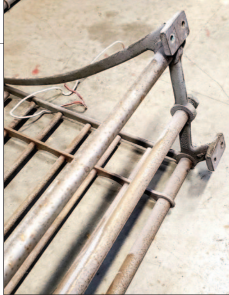
▲ The rusty luggage racks were stored awaiting the budget to have them stripped and recoated with nickel. Paul Averdung later said the process of reinstalling the racks was like assembling a 1,000-piece jigsaw puzzle, since the racks had to be completely disassembled into individual rods and brackets for stripping and recoating.—Eric Zabelny photos
