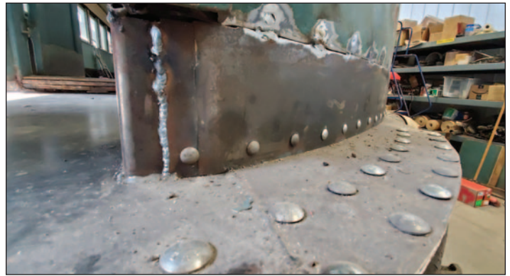
▲ These photos both show one of the west end center posts of the car, with extensive corrosion and rot (left), and with new steel welded in place (right).—Eric Zabelny photos
