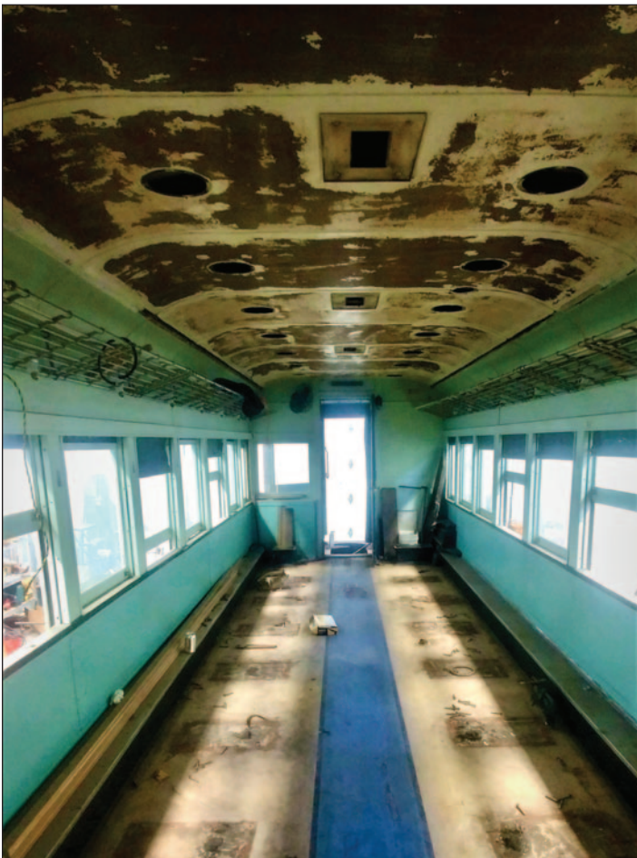
▲ Left: The seat bases, heat registers and all interior lighting fixtures have been removed in this photo. Many hours of needle scaling the ceiling would be needed to achieve a bare metal surface. Right: After priming and painting, the ceiling looks brand new!—Eric Zabelny photos
