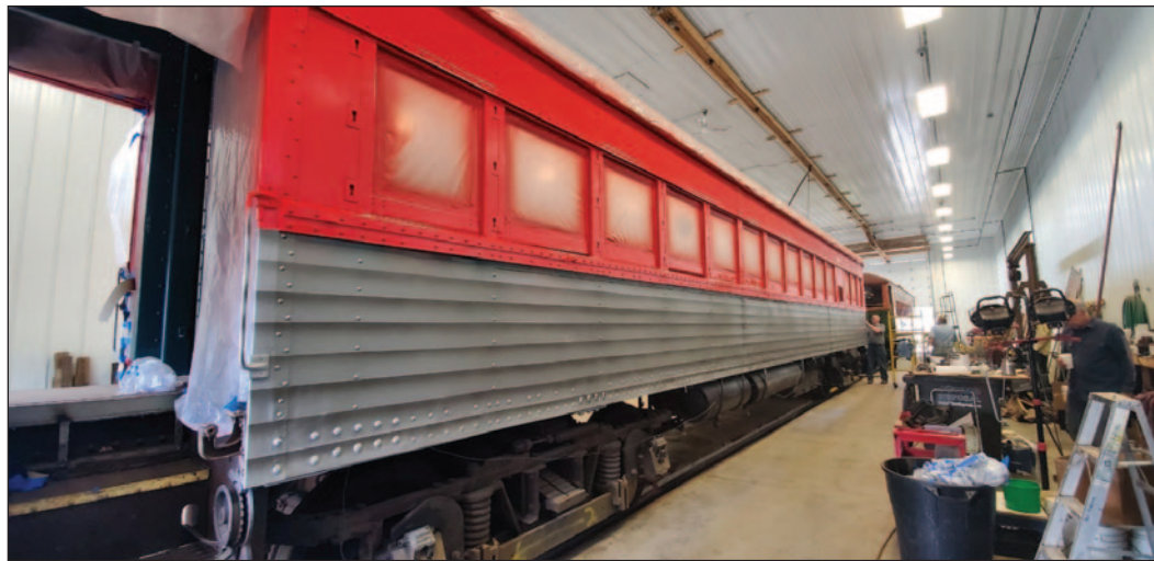
▲ The tape had just been removed, revealing the terrific job done by Eric and Paul to recreate the stainless-steel appearance used by the North Shore line in the 1950s to modernize the look of their cars. You had to touch the car to make yourself believe that it wasn’t fluted stainless-steel.— Eric Zabelny photo
