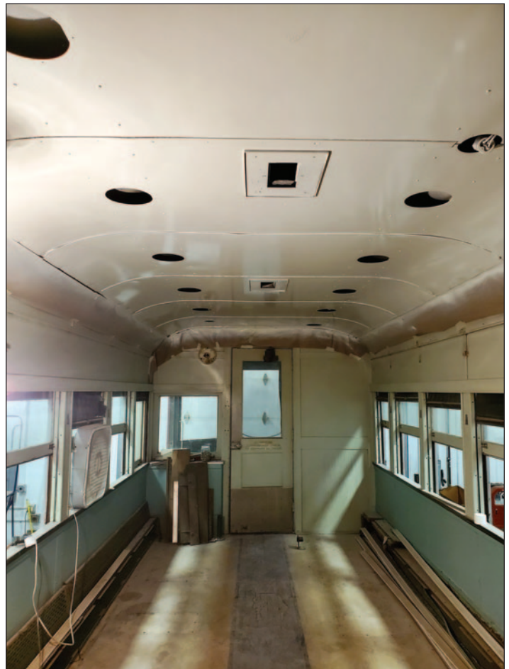
▲ Left: The seat bases, heat registers and all interior lighting fixtures have been removed in this photo. Many hours of needle scaling the ceiling would be needed to achieve a bare metal surface. Right: After priming and painting, the ceiling looks brand new!—Eric Zabelny photos
