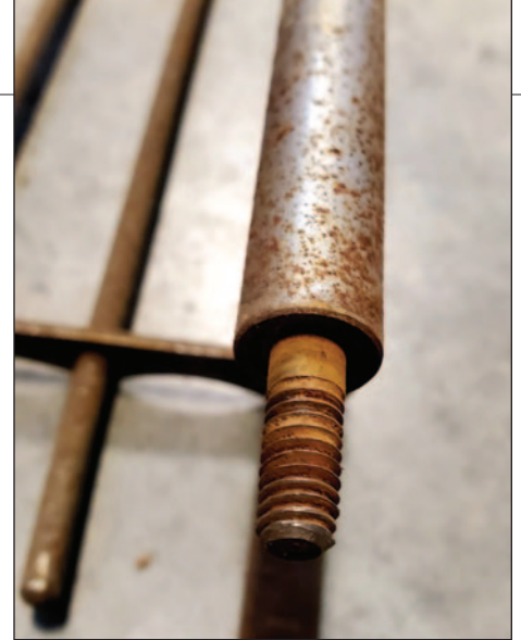
▲ The rusty luggage racks were stored awaiting the budget to have them stripped and recoated with nickel. Paul Averdung later said the process of reinstalling the racks was like assembling a 1,000-piece jigsaw puzzle, since the racks had to be completely disassembled into individual rods and brackets for stripping and recoating.—Eric Zabelny photos
