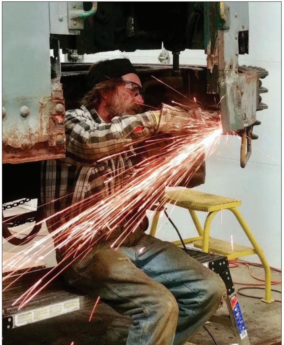
▲ Mike Heck cuts away rotted steel sections in this photo by Eric Zabelny.
