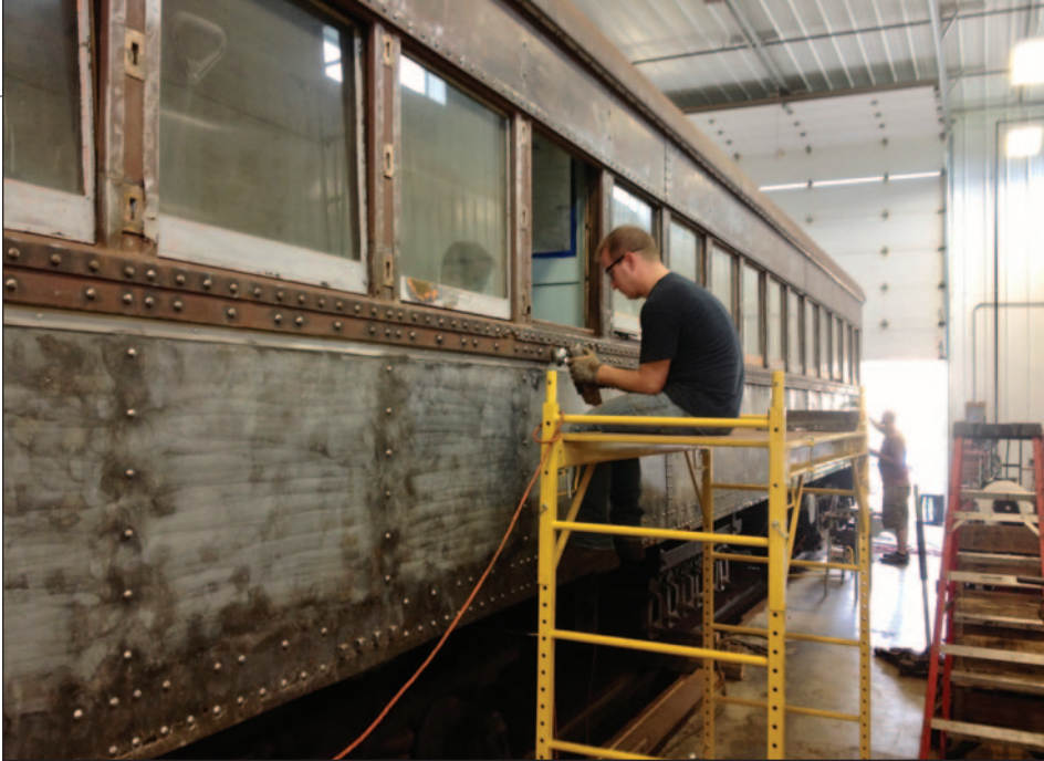
▲ Eric is hard at work grinding rust off of every nook and cranny of the body of the car. This was the most tedious part of the project for him and took three times as long as he estimated it would take.
