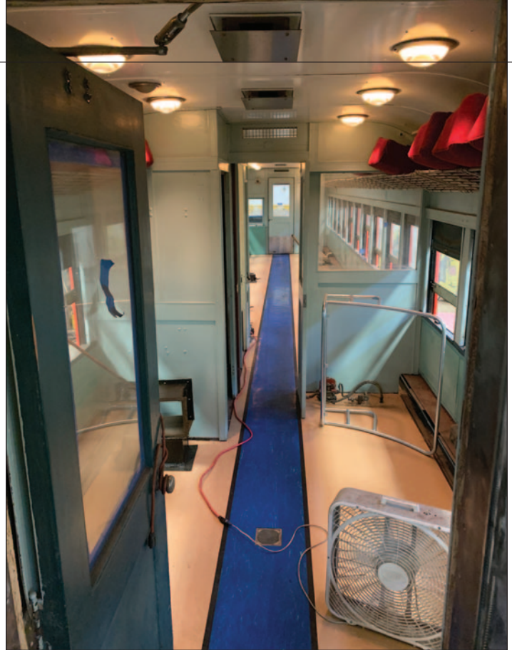
▲ In early January 2021, the interior of the car had been painted, the lighting fixtures and vent hardware had been reinstalled, the luggage racks were in place, and some of the seat mounting bases had been installed. One seat frame and several reupholstered cushions are visible in this photo. We purchased the flooring from the same company that made the flooring for the North Shore Line in the 1950s.
