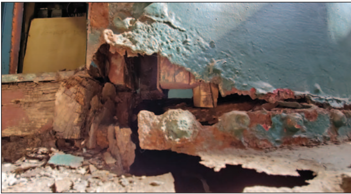
▲ These photos both show one of the west end center posts of the car, with extensive corrosion and rot (left), and with new steel welded in place (right).—Eric Zabelny photos
