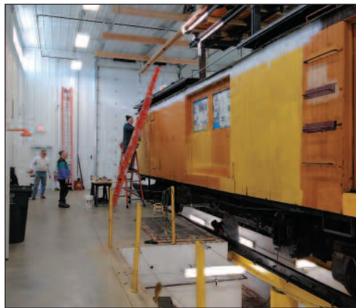
▲ Jerry Borzych, on the ladder, works to prime wood siding that has been repaired or replaced. Steve Southworth and Joe Buerger look on. —East Troy Railroad Museum Photo Archives ▲ Joe Buerger (left) and Mike Jaehn attach new trim to the car. —Ryan Jonas photo
