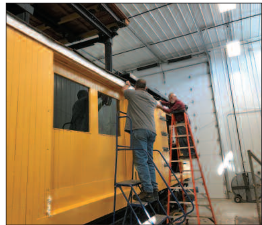
▲ Jerry Borzych, on the ladder, works to prime wood siding that has been repaired or replaced. Steve Southworth and Joe Buerger look on. —East Troy Railroad Museum Photo Archives ▲ Joe Buerger (left) and Mike Jaehn attach new trim to the car. —Ryan Jonas photo
