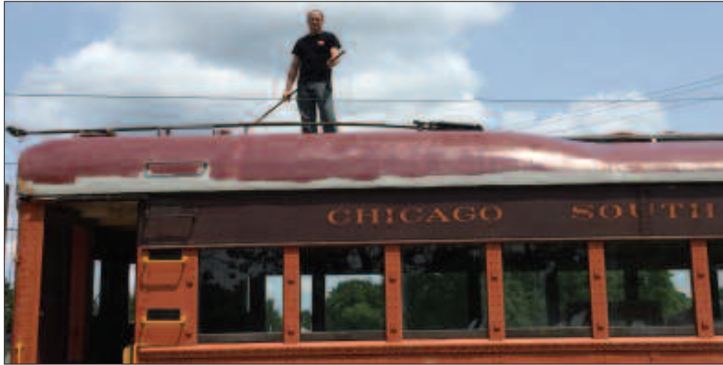
▼ Ryan Barry is shown on top of CSS&SB car 9 re-staining the roof. —Ryan Jonas photo
