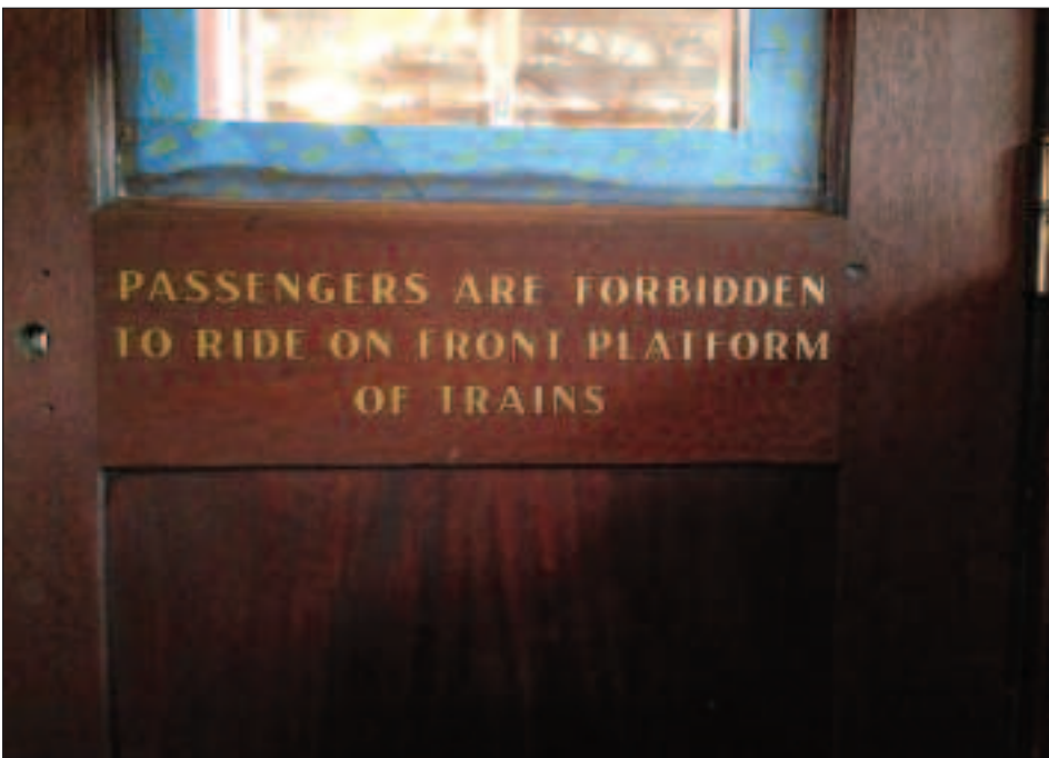
▲ Decals were created to match the original lettering at the end doors of the car. They were applied and then coated with a thin layer of polyurethane.
