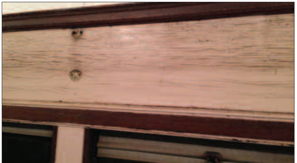
▲ After removing the luggage racks, the color of the original wood could still be clearly seen. The shellac had deteriorated and cracked, but Barry could see the original color. His goal became matching the original color and finish.
