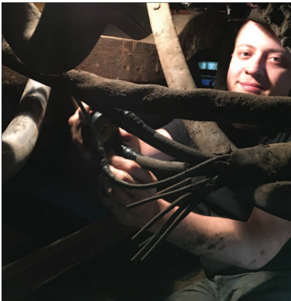
▲ Car 33's "new" air compressor has been repaired and tested and is ready for installation. This large compressor is so heavy that it could only be moved with the assistance of a forklift attached to the railroad's front end loader. ▼ Ryan Barry works beneath the car to splice and tape some of the wiring that had been cut when the car was being cosmetically restored in Indiana.
