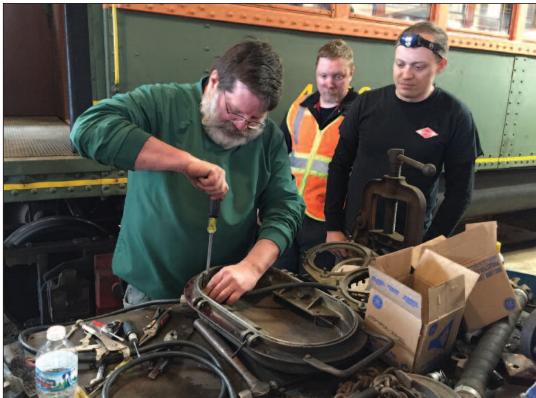
▲ Both control stands were removed, disassembled, cleaned, rewired and lubricated before being reinstalled in car 33. ▼ Volunteer Ben Killips works to repair and reassemble one of the “new” headlights for car 33, while Dustin Robinson and Ryan Barry look on.
