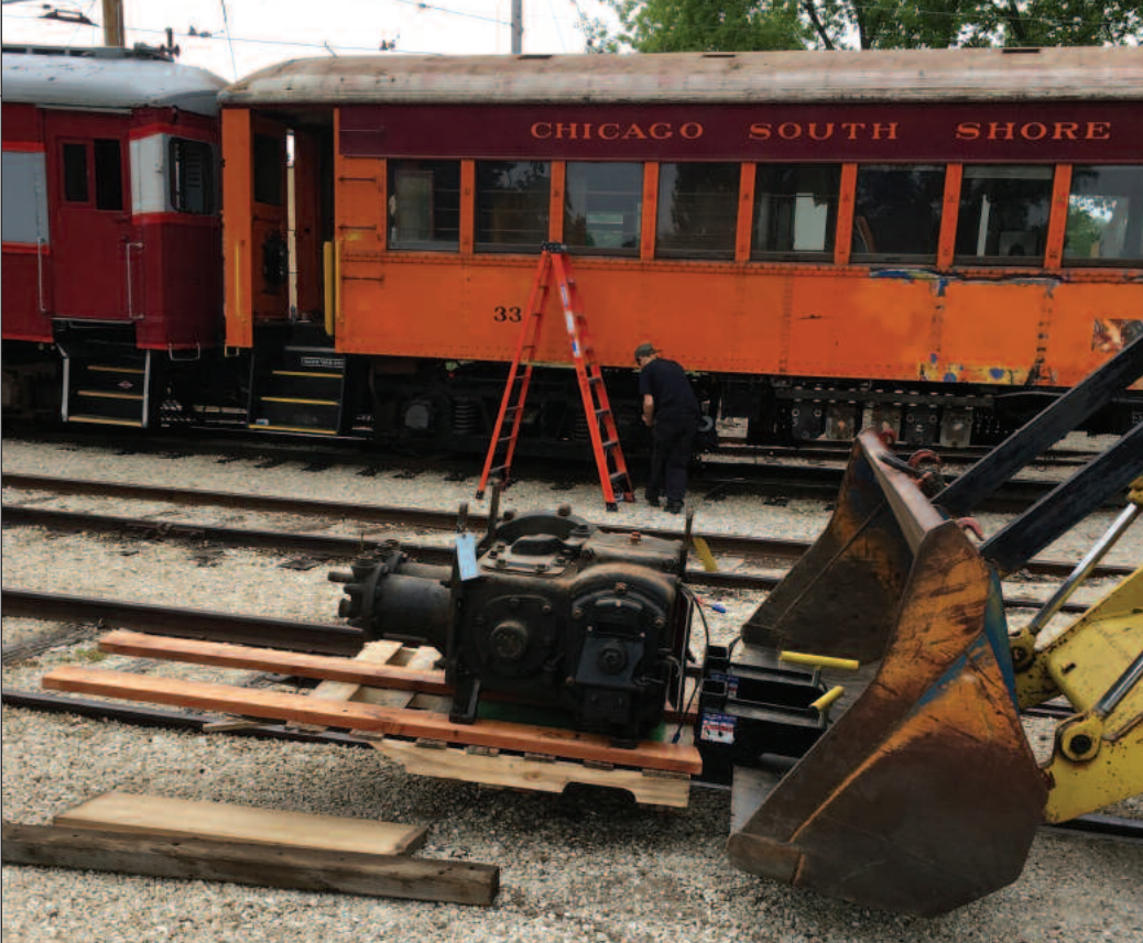
▲ Car 33's "new" air compressor has been repaired and tested and is ready for installation. This large compressor is so heavy that it could only be moved with the assistance of a forklift attached to the railroad's front end loader. ▼ Ryan Barry works beneath the car to splice and tape some of the wiring that had been cut when the car was being cosmetically restored in Indiana.
