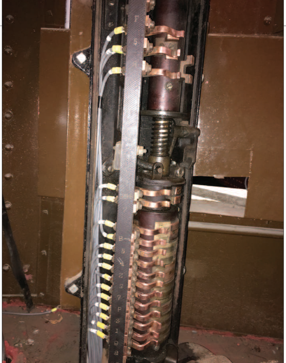
▲ Both control stands were removed, disassembled, cleaned, rewired and lubricated before being reinstalled in car 33. ▼ Volunteer Ben Killips works to repair and reassemble one of the “new” headlights for car 33, while Dustin Robinson and Ryan Barry look on.
